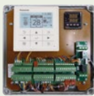
PCB, Power trans, Terminal block
